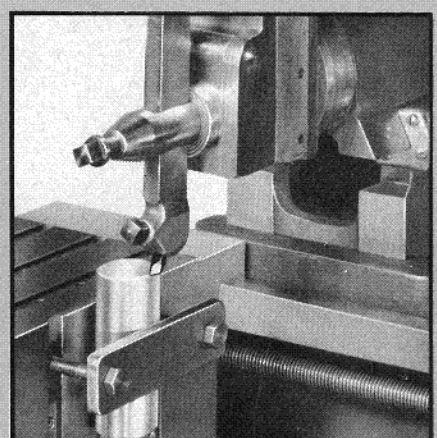
Machining end of round piece of work held in "V" groove on side of table.
