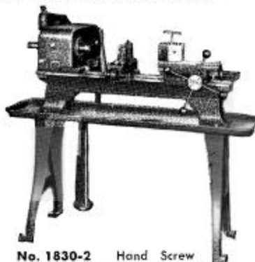
No. 1830-2 Hand Screw Machine. 43" bed, Pilot Wheel Turret, V-Belt drive. Lever operated double tool post cross slide clamps directly to bed in place of carriage.
